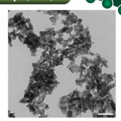
• These TEM photographs indicate the fact that the nanocrystalline HAp particles prepared by the microwave assisted synthesis has rod-like shape of 80-93 nm in length with a diameter of 8-14 nm (scale bars: 100 nm).
